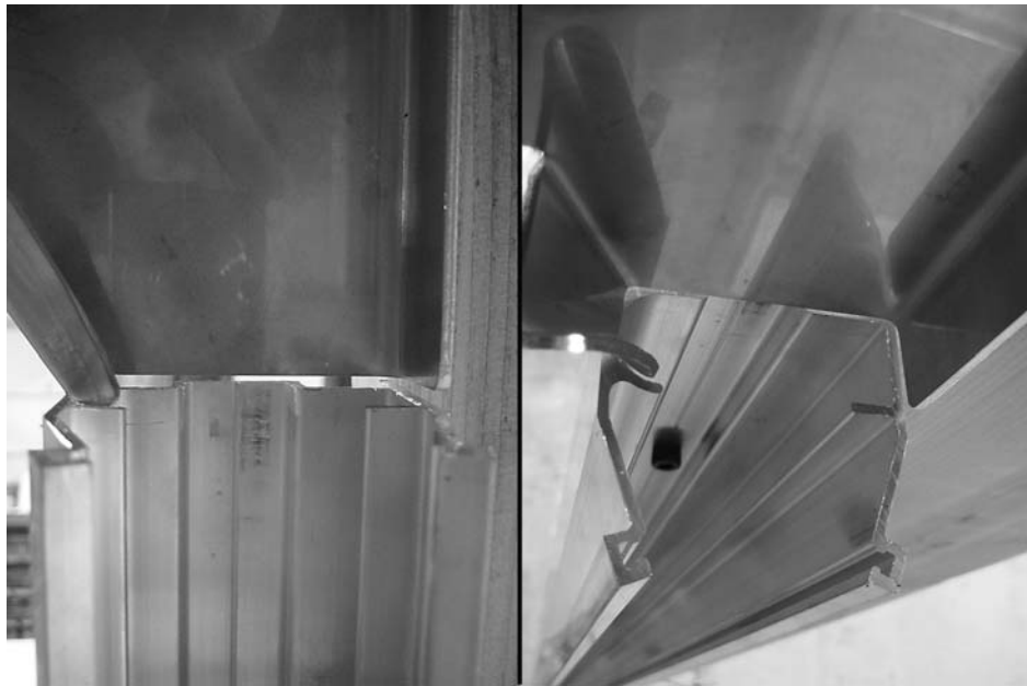
Photo #1 (Bracket to Extrusion Alignment)
